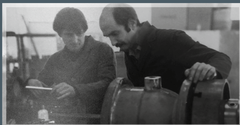
Valve machining with an horizontal lathe 1978
