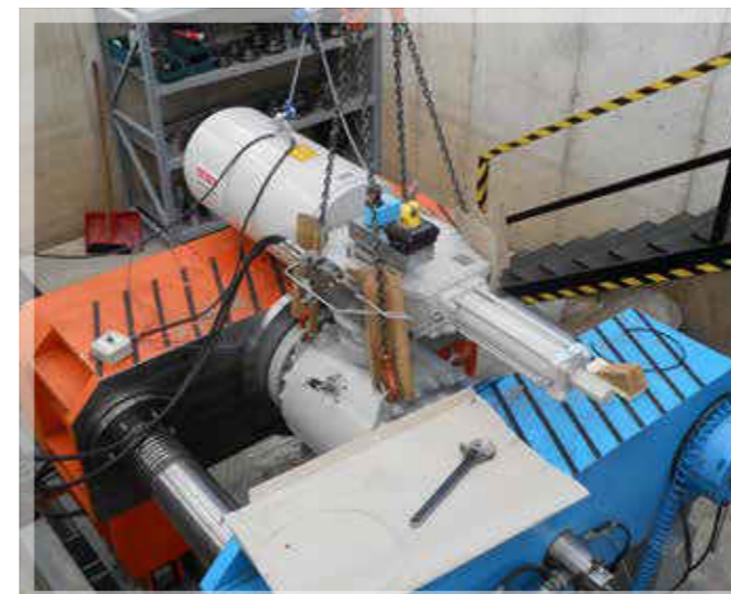
Valve & Actuator Factory Acceptance Test acc. to Client specification
