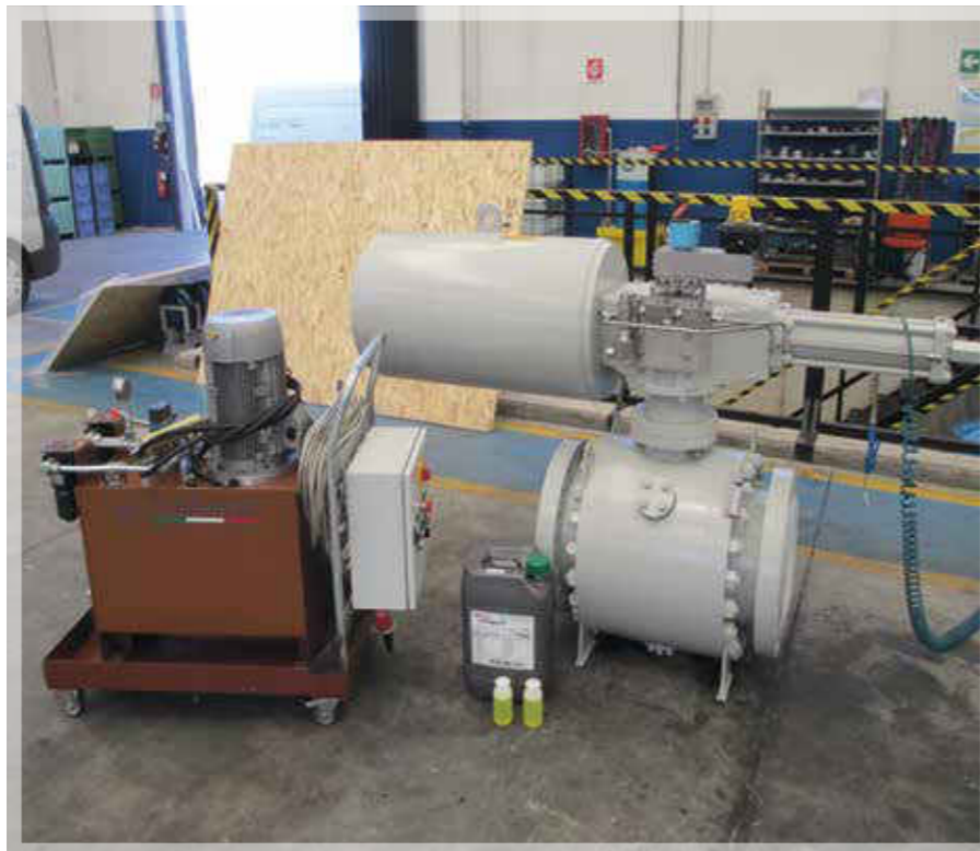
Actuator Flushing / NAS Cleaning
