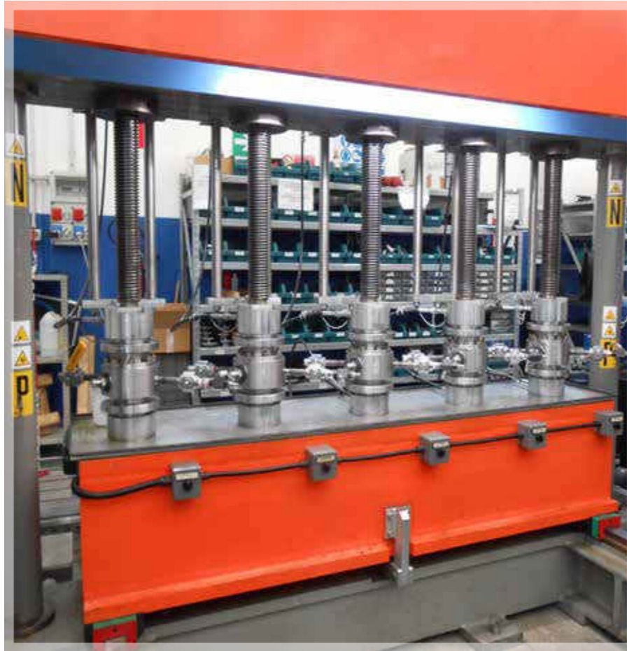
Multiple Stations Test Bench ( Hydrostatic and Gas Test )
