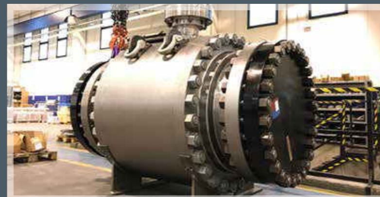
36" 600 class ball valves ready for test
